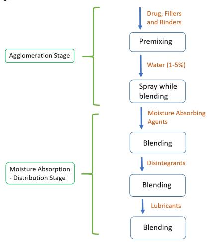
**Fig. 2.** Step-wised flow diagram of the MADG process.
