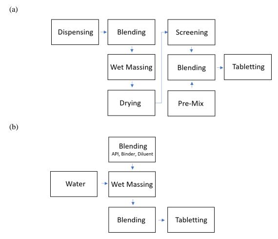
Fig. 1. Process steps involved in (a) traditional wet granulation, (b) the MADG<sup>3</sup>.
