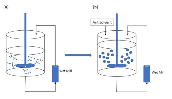
Figure 2. The Schematic Process Flow Diagram of CPT
