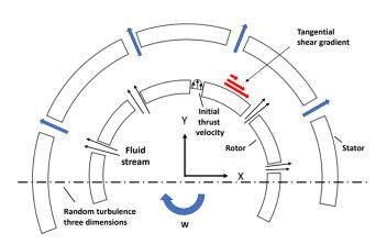
Figure 5. Schematic representation of hydrodynamics of fluid in a toothed rotor-stator device
