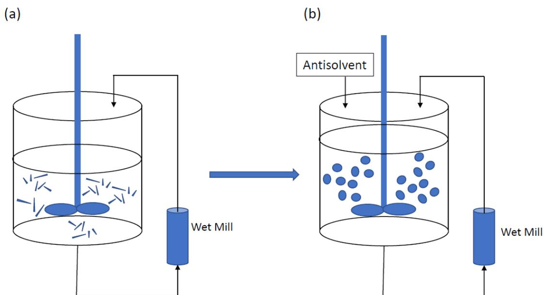
Figure 2. The Schematic Process Flow Diagram of CPT
