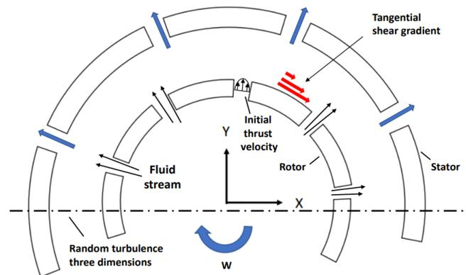
Figure 5. Schematic representation of hydrodynamics of fluid in a toothed rotor-stator device
