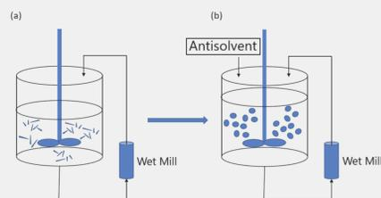
Figure 1. The Schematic Process Flow Diagram of CPT
