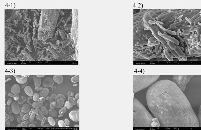
Figure 4. SEM analysis for 4-1) As-received API X (\*300), 4-2) As-received API X (\*2000), 4-3) CPT API X Product (\*300), 4-4) CPT API X Product (\*2000)
