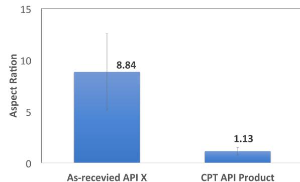
Figure 3. Aspect ratios of As-received API X and CPT API X product.
