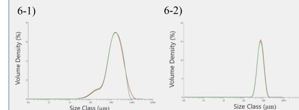
Figure 6. Particle Size Distribution of 6-1) As-received API X and 6-2) CPT API X product.
