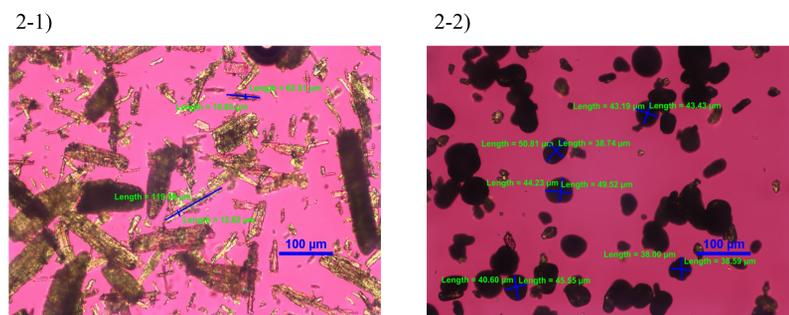
Figure 2. 2-1) shows an example of PLM image of as-received API X and 2-2) shows an example of PLM image of the CPT API X product.
